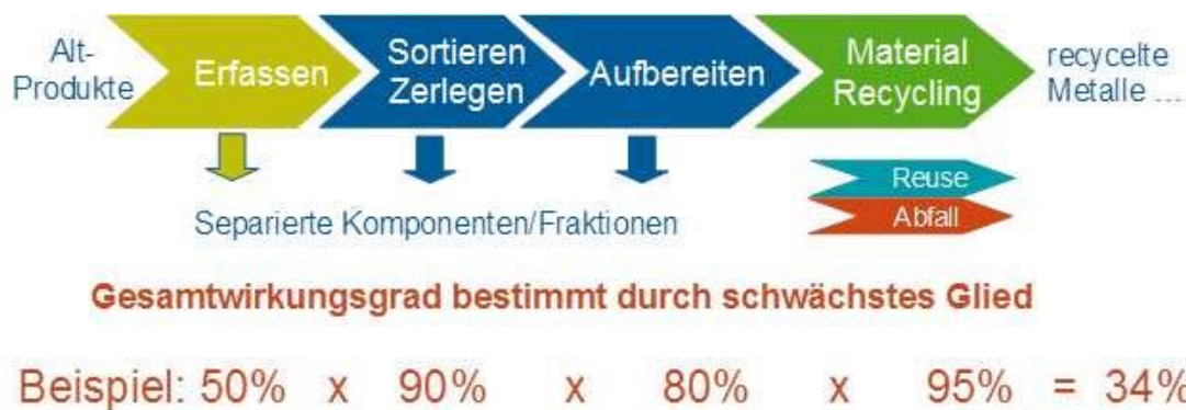
Figure 41 Typical efficiency of high-tech metal recycling chain [Hagelüken, Treffer 2011]
